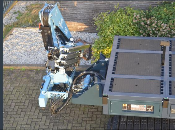
Versatile Crane Booms, by means of two knuckle booms, Crane Boom rotation and impressive Telescopic boom. Fully proportional controlled and each Crane function operated by a dedicated joystick controller.
